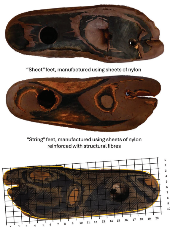
Figure 4: The two type of feet manufactured by the JJCDR (top) and plantar surface of a prosthetic foot (bottom) with a grid.
